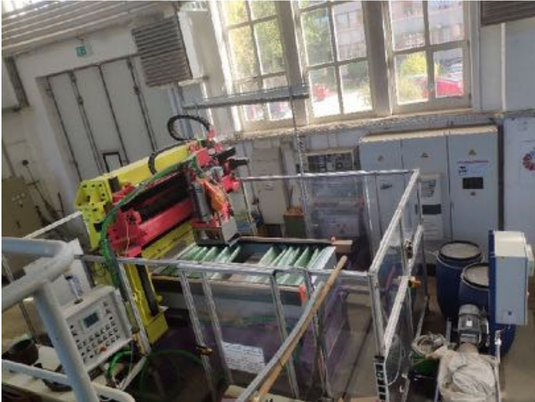
Cutting test rig at TUBAF: A water filled box with rock material, the green cover is for splashback
